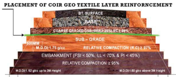
Fig.1. Typical Road cross section
