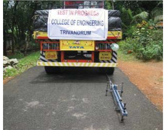
Fig.5. Benkelman beam test in progress
